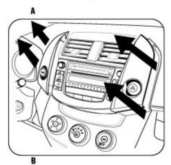
3 Remove (4) 10mm screws securing the radio. (Figure B)
